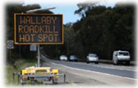
Figure 8-Variable Message Sign during the day
