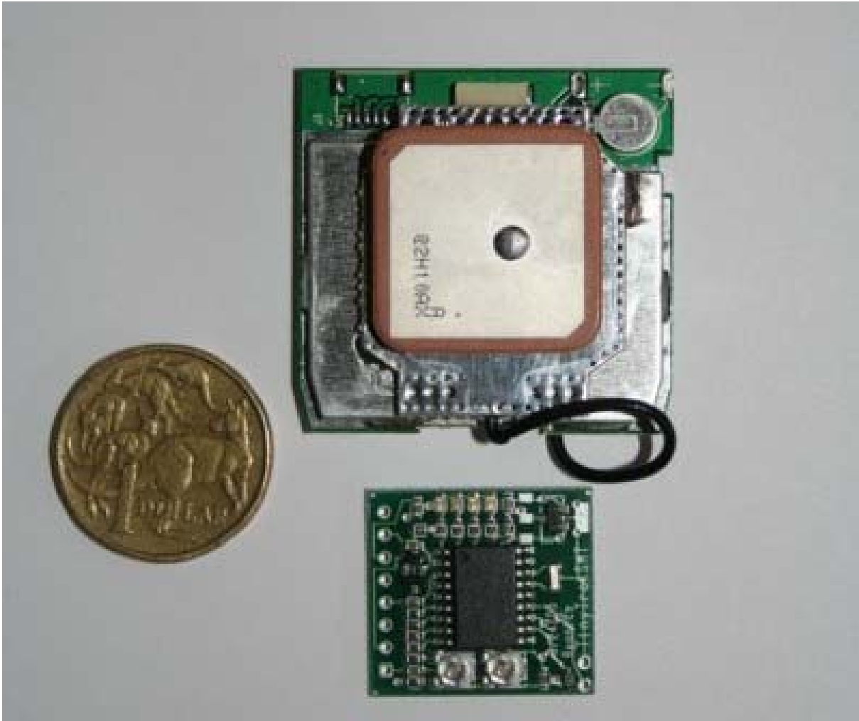
Figure 2 APRS components, GPS above and smart encoder below. Radio transmitter and batteries not shown.
