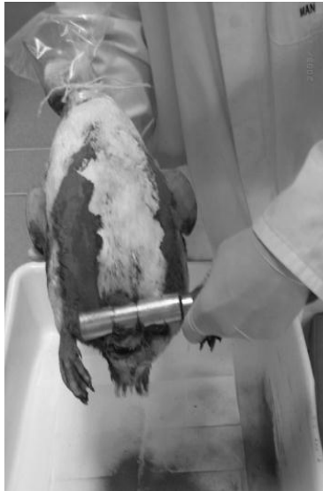
Figure 1: The removal of contaminant-laden magnetic particles from the plumage of an oiled Little Penguin ( Eudyptula minor ) carcass utilizing a magnetic harvesting device.
